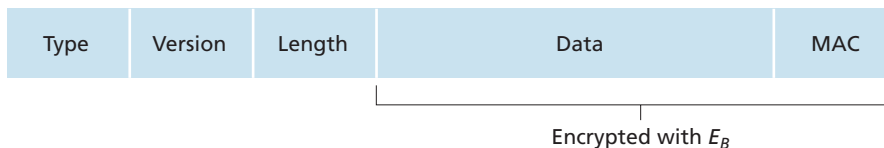
Figure 8.26 ♦ Record format for SSL
