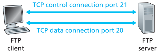
Figure 2.15 ♦ Control and data connections
